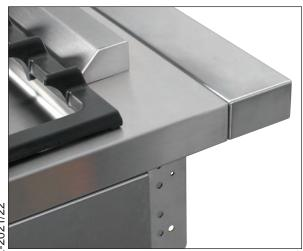
With the back infill panel in place, a 70 mm space remains between the range and the wall. The overall depth of the appliance (rail not included) then reaches 720 mm (an increase of 70 mm). The back infill panel prevents excessive heat transfer to the wall and makes cleaning easier. It is especially recommended for all ranges equipped with gas ovens or those with tiles on the wall above the cooker.
